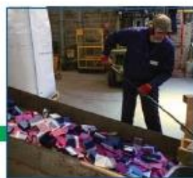
TipOne® refill wafers and racks going into the granulator
